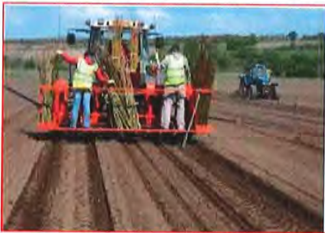
A “Step Planter” automatically cuts the willow rods into short lengths and plants them at precise spacings throughout the cultivated area.
