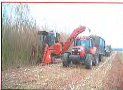
A Case IH (Austoft) billet harvester working SRC willow. (billets are pieces of wood 5 to 20 cm long. In Billet heaps, unlike wood chips, air can circulate and dry out the biomass. Wood chips immediately start to heat up and decompose)
