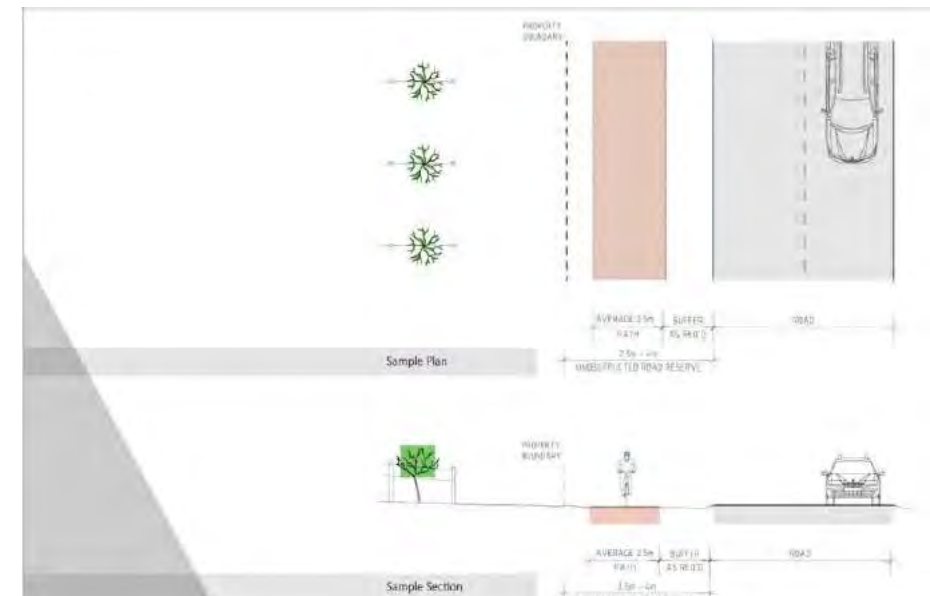
Figure 11. Schematic drawing of off-road treatment beside a road within a road reserve.
