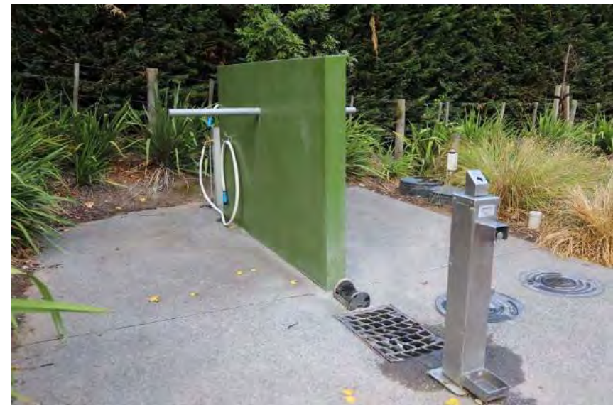
Figure 20. Wash and repair station incorporating repair stand, wash down hose, boot cleaning and drinking fountain with dog bowl.
