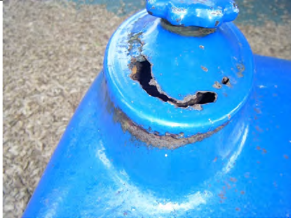
Rusted sharp edges
