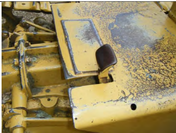
Crush point, sharp edges, finger entrapment
