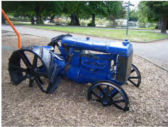
Head entrapment gaps, sharp edges
