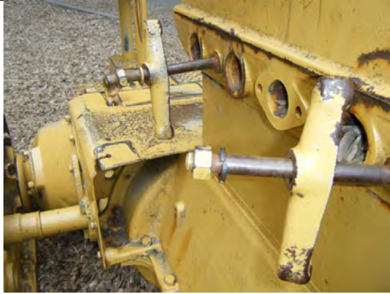
Finger entrapment gaps, protrusion and sharp edges
