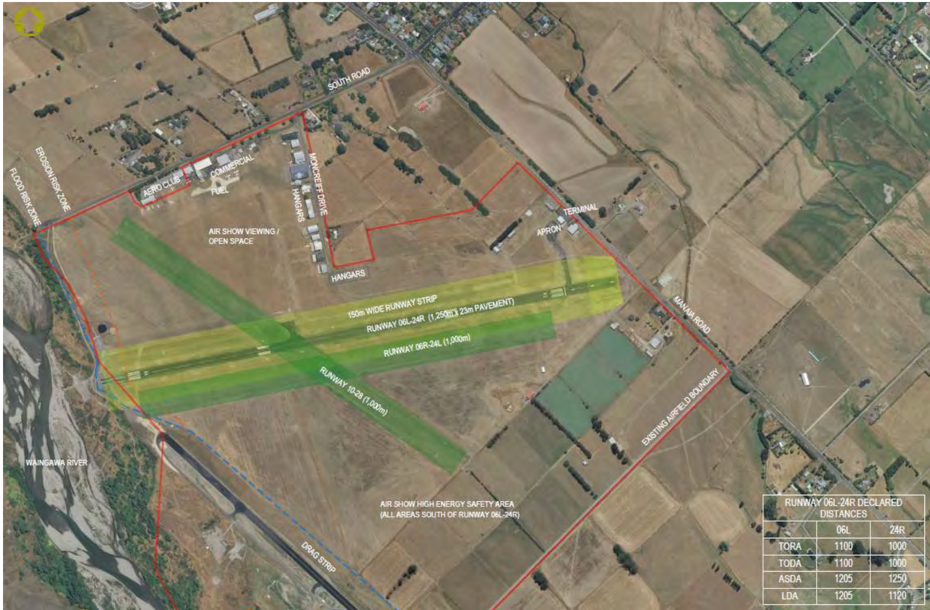
Figure 2 - Existing airfield layout
