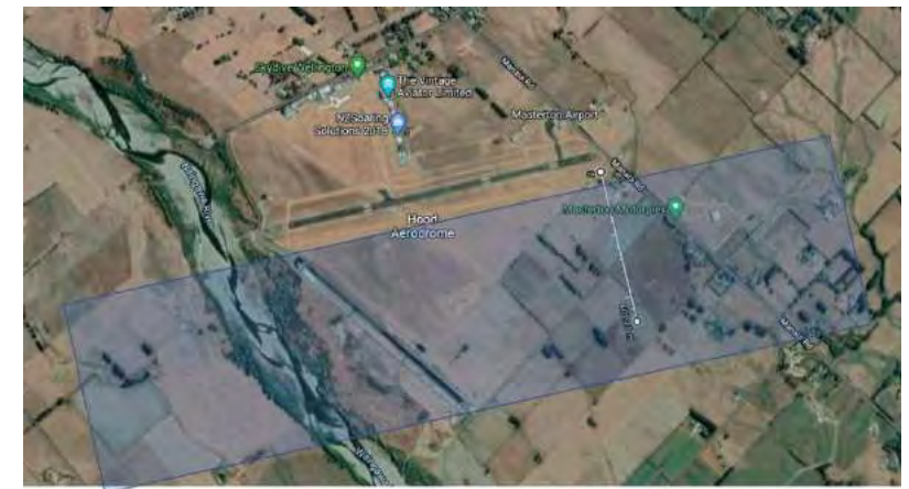
Figure 7 - High energy safety area shown in blue
