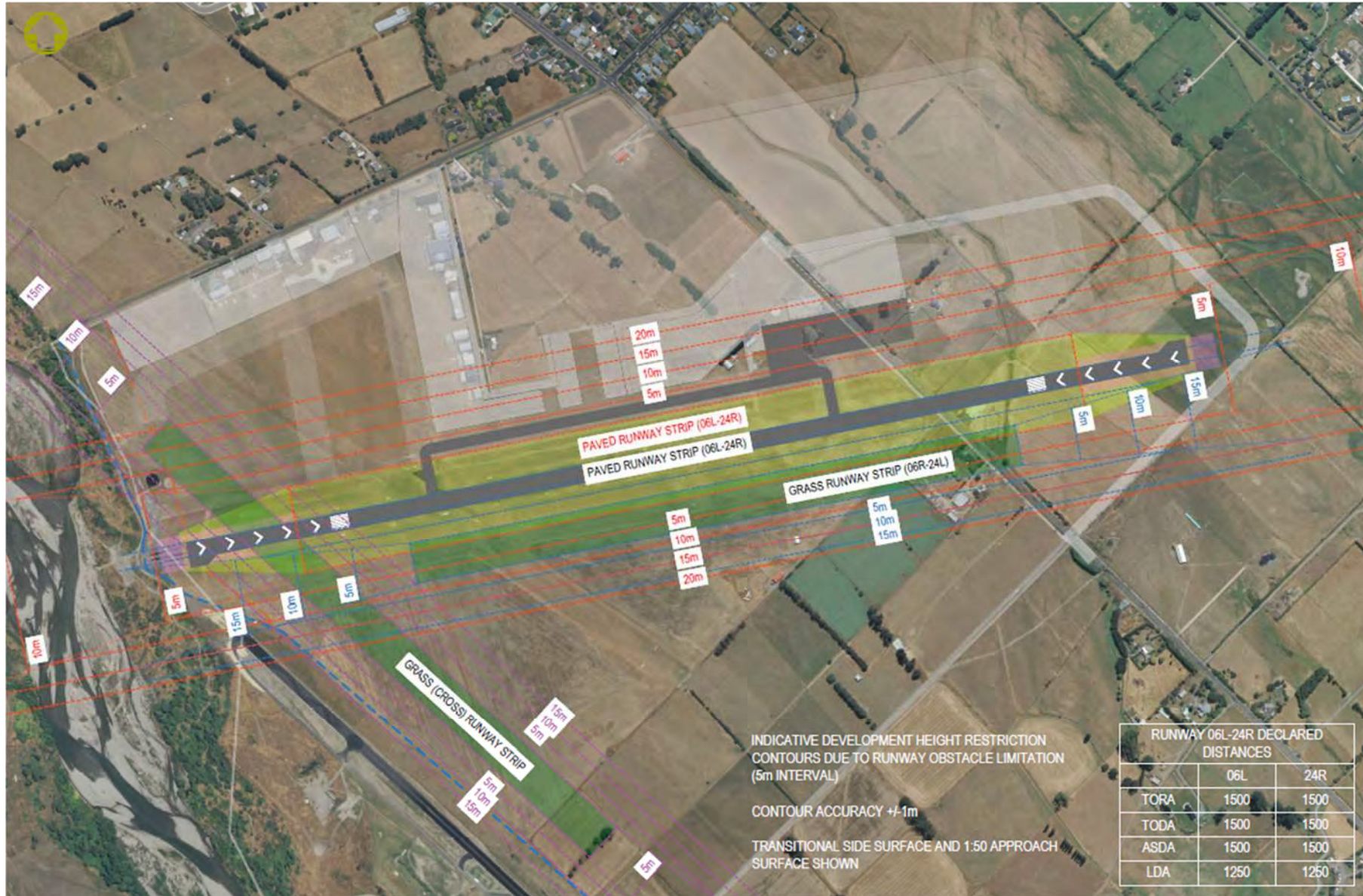
Figure 16 – Proposed runway system including Indicative development height restriction contours due to runway obstacle limitation surfaces.
