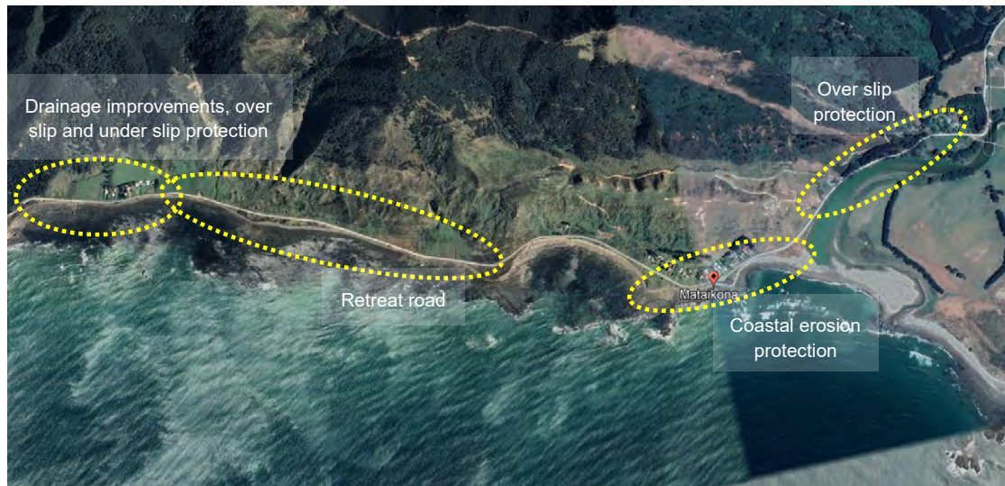
Figure 2-7: Middle settlement to Mataikona and preferred interventions
