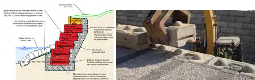
Figure 6-9: Example Hybrid Wall using Concrete Block Wall with Armour Revetment (Redi Rock, 2023)
