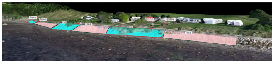
Figure 6-5: Middle Settlement (red areas of top-up to current fix , cyan indicates full coastal protection installation)
