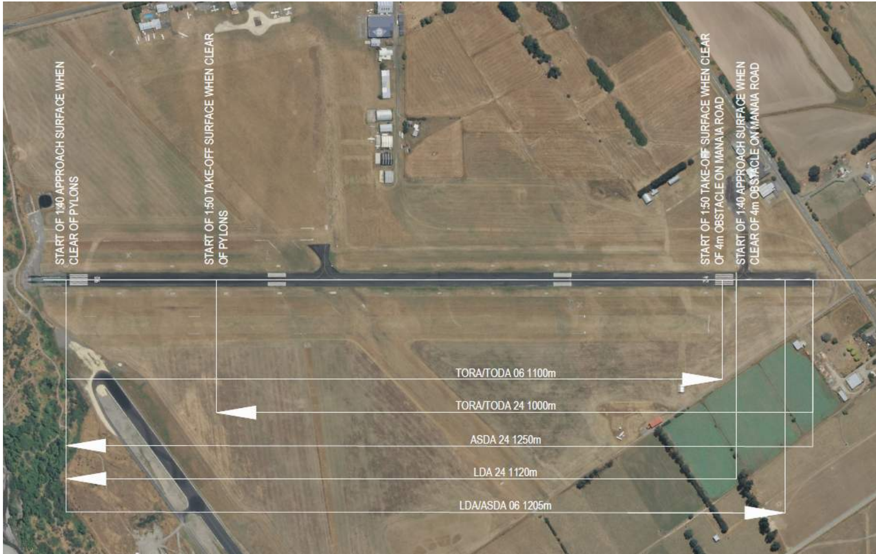
Figure 10 – Existing (as of 2021) Runway 06-24 declared distances
