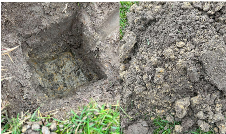
Photo 1 and 2: Typical 3s1 soil profile. Mottled Pallic soil with dense clay fragipan at the bottom.
