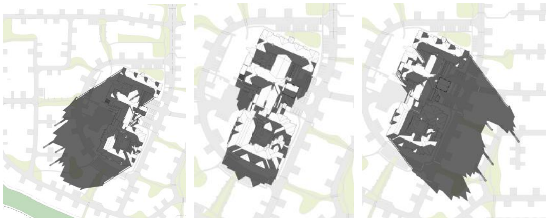
Figure 3, 4 and 5: Shadow Diagrams for the main building on the shortest day in Winter.
