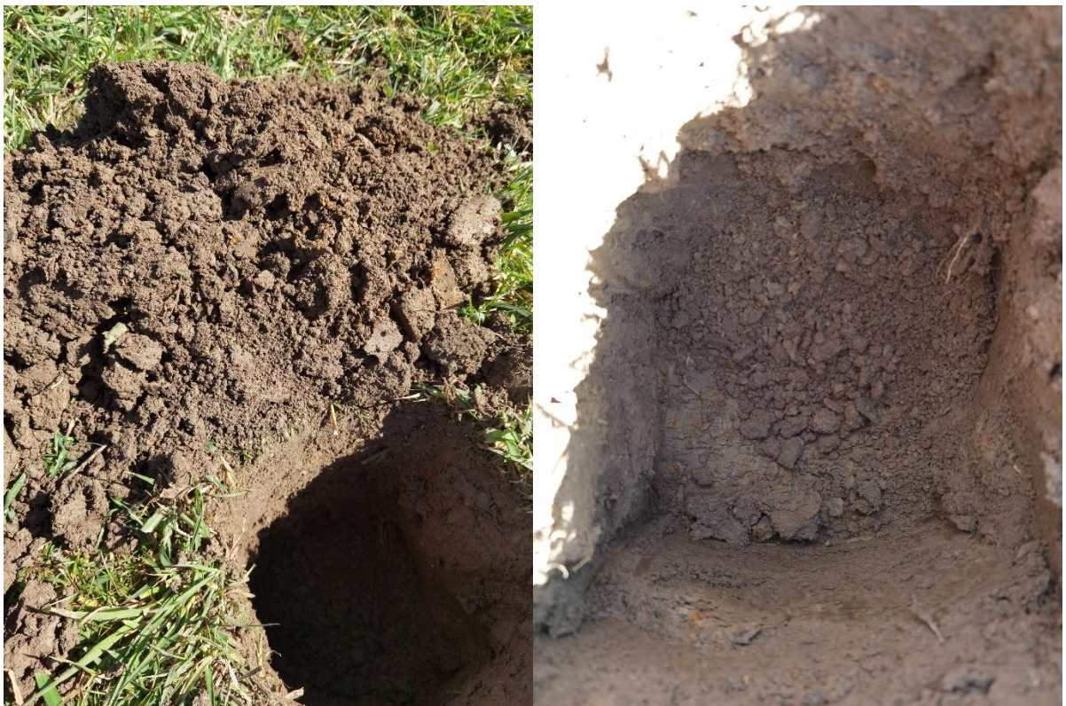
Photo on left showing topsoil and some mottling from subsoil and on the right showing the hard subsoil and mottling.
