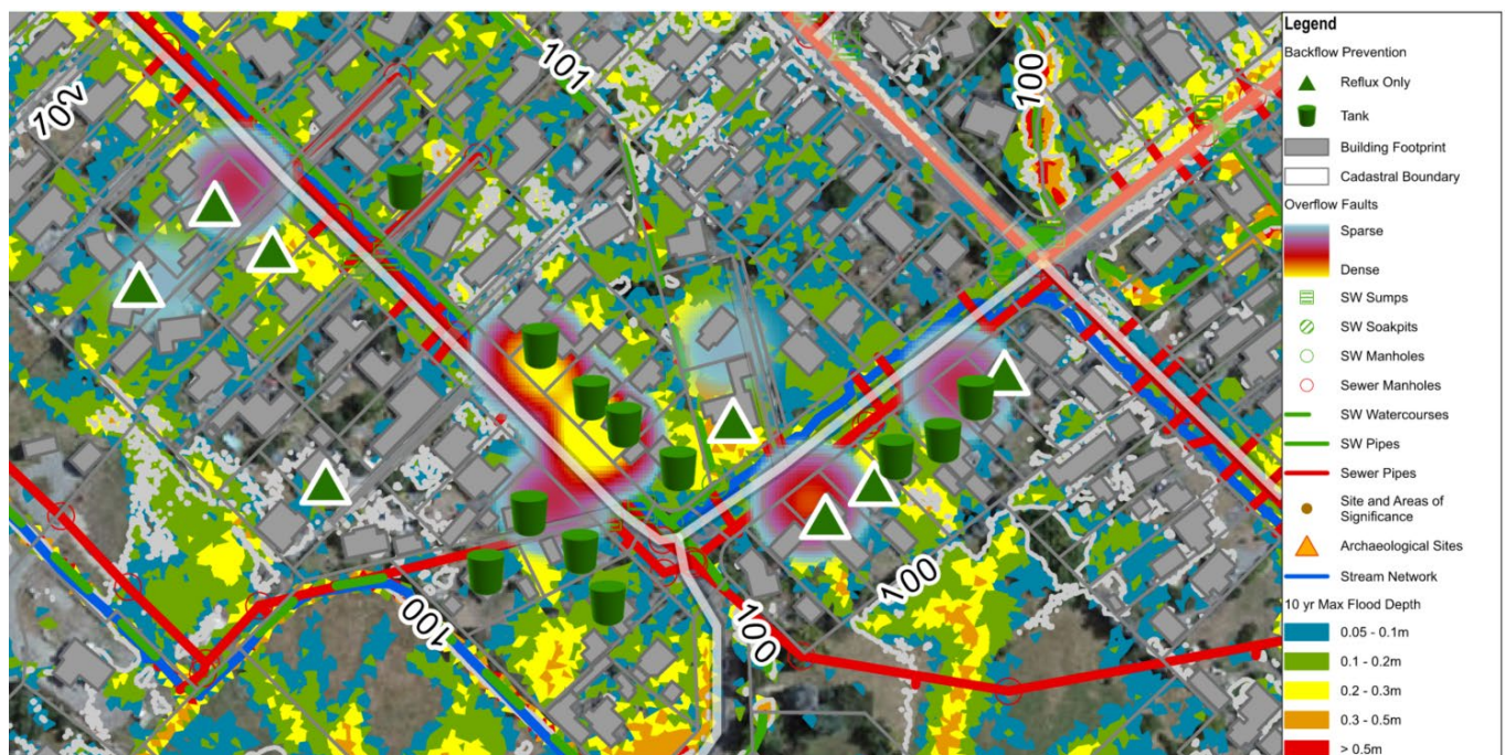
Figure 7 Reflux valves and tanks installed at Cockburn/Colombo St (extract from Appendix A, tank at 129 Makoura Road not shown)
