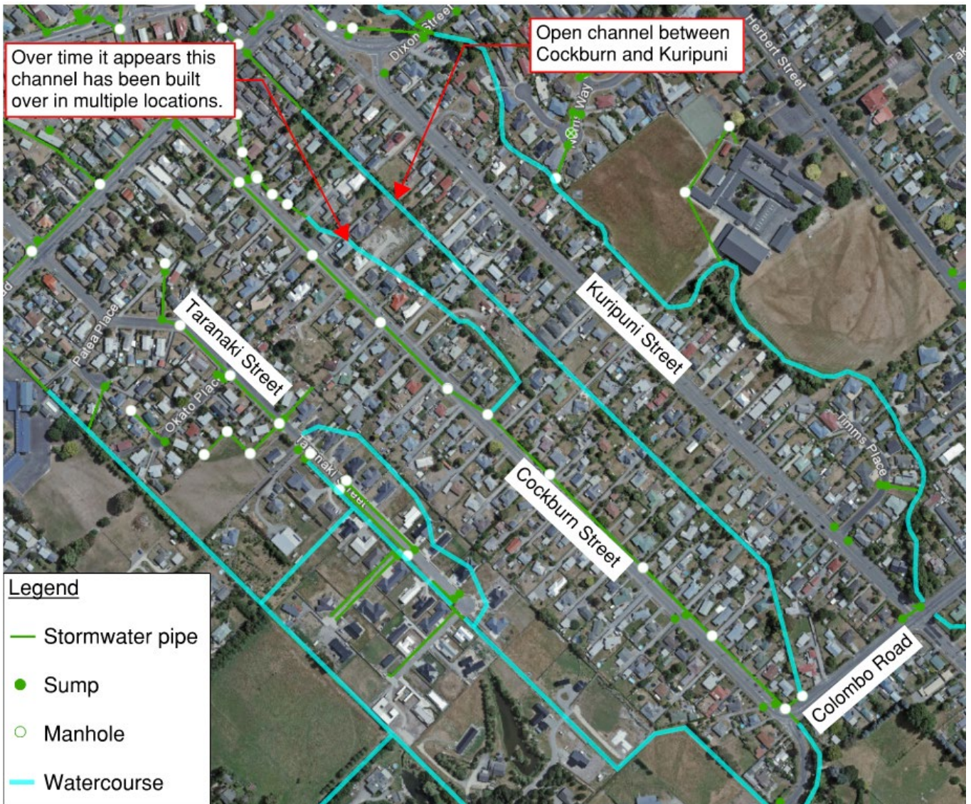
Figure 5 Stormwater network and watercourses in and around the Cockburn catchment (Wairarapa Maps GIS)
